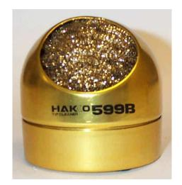
plunge the tip into the coiled wire. The wire is softer than the tip plating yet harder than the oxidation that forms on the tip. The 599B tip cleaner may be used in lieu of a damp sponge.
